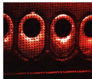
At the Scheimpflug angle, the entire surface becomes focused.
