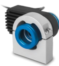
LTPRUP-x models for strobe-only operation featuring ≈ 90W peak power intensity. These models are compatible with CMH0016 clamping mechanics, alternatively three M4 and one M6 threads are available as fixing options.
