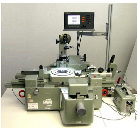
Refurbished X-Y measuring microscope
