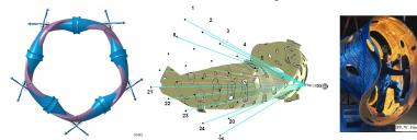
Layout design of Wendelstein 7-X video diagnostic system with 30° FOV objective and chamber during manufacturing process
