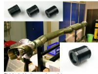
Finished objectives and complete diagnostics tube with objectives inside in
